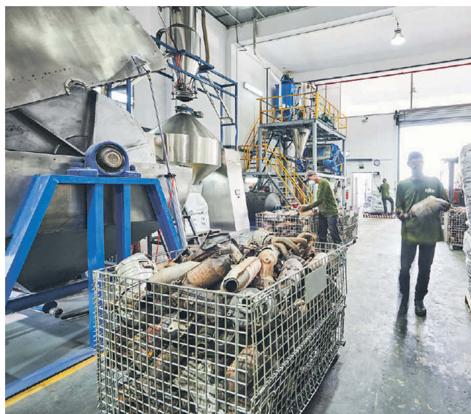
Parts like catalytic converters found in vehicles are efficiently recycled, and metals like platinum and rhodium are extracted as a result. PHOTO: BR METALS
